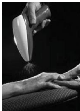
Figure 14. battery-operated hand-held electrospinning apparatus [69].
